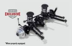
**2500** THE AVAILABLE AUTO-LEVEL REAR AIR SUSPENSION SYSTEM takes its engineering cues from the available Ram I500 Active-Level™ Four-Corner Air Suspension System. This Ram Heavy Duty adaptation addresses needs specific to the higher GVWRs and GCWRs of the 2500 class. The two modes: Normal Load-Leveling Mode, which provides a level load profile; and Alternate Ride Height Mode, which keeps an even alignment between the hitch and trailer tongue.
