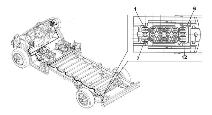
Chassis Harness Connector – Tyco P/N 284844-1 Tail Light Harness Connector – Tyco P/N 254848-3
