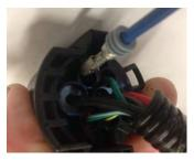
Re-install the lock and re-attach the harness connecter to the trailer connector
