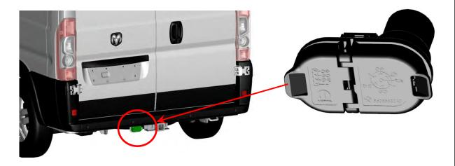
The AA and AB versions do not have provisions for the trailer brake circuit. MOPAR is releasing an "AC" version that will have the brake control wire in the harness. That kit should be available early in the third quarter of 2014.
