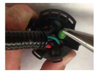
Insert the wire with terminal into the back of the connector, when fully seated, you should not be able to pull the terminal back out
