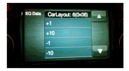
6. Touch the line for **+1** or **-1** to scroll through the different layouts until the desired layout appears in the top line. For enabling rear speakers, select 8(0x08).
