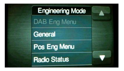
10. Exit the **Engineering Mode** menu by pressing the **RADIO** and **MEDIA** buttons then, shortly after that, while still holding **RADIO** and **MEDIA**, press the **BROWSE/ENTER** button. Hold all for approximately 5 seconds. The normal Radio or SXM tuning screen will appear.
