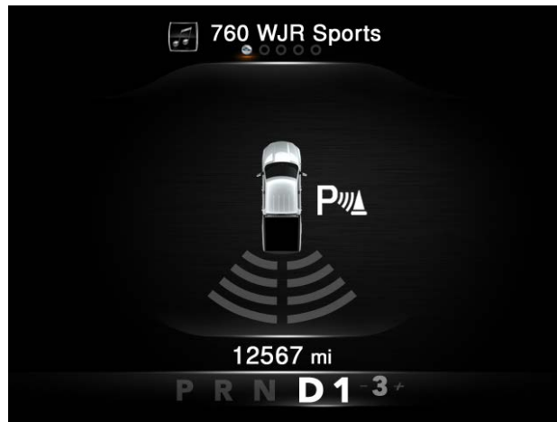
Figure 13: Instrument Cluster Graphic with no obstructions detected (Highline Cluster Left – Midline Cluster Right)
