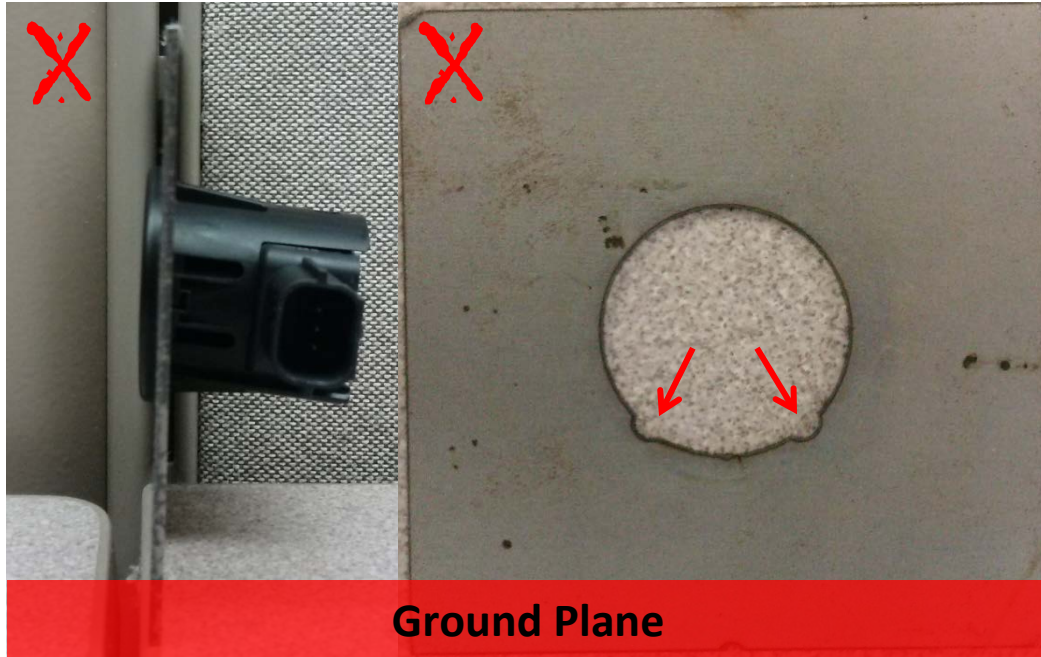
Figure 6: Incorrect coupon and Sensor Mounting
