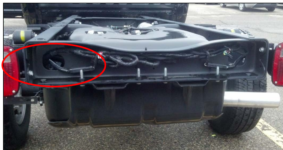
Figure 8: Factory ParkSense Connector Location
