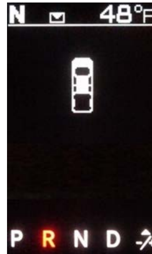
Figure 13: Instrument Cluster Graphic with no obstructions detected (Highline Cluster Left – Midline Cluster Right)
