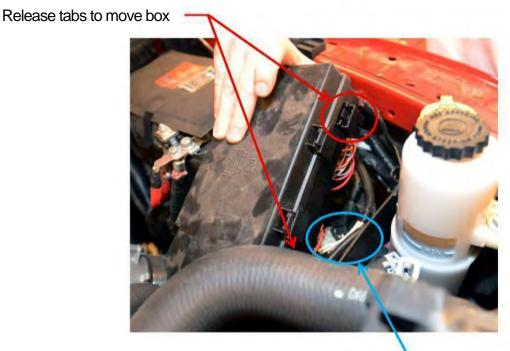
Wires located in front of PDC
