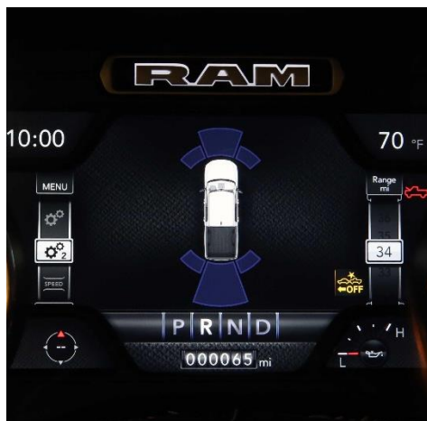
Figure 12 Instrument Cluster Graphic with no obstructions detected (High-line Cluster Left – Mid-line Cluster Center – Low-line Cluster Right)
