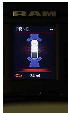
Figure 12 Instrument Cluster Graphic with no obstructions detected (High-line Cluster Left – Mid-line Cluster Center – Low-line Cluster Right)
