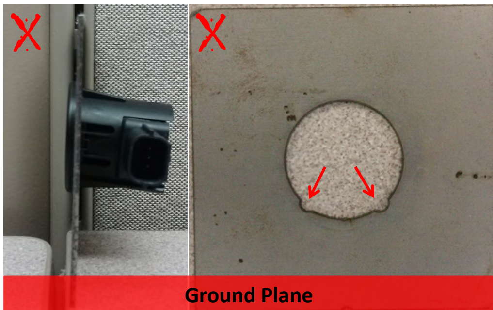
Figure 6: Incorrect coupon and Sensor Mounting
