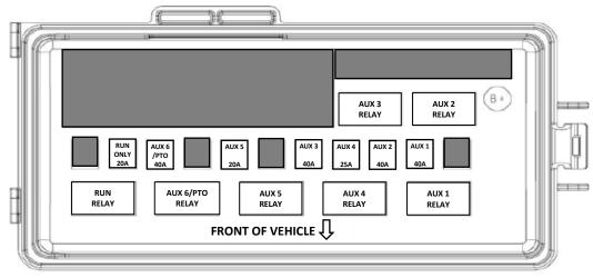
Max Combined Fuse "rating" allowed for Aux Switches 1,2,3,4,5,6 and Run Only is 225A. These Aux/PTO/Run fuses can be relocated to accommodate the loading on them. The maximum allowable total continuous amperage is 135A. Maximum fuse rating in any one location is 40A.
