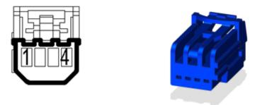
The control circuit that should be spliced into is K321. It goes between the body controller and pin 3 of the BTSI connector. The body controller fires the solenoid when the service break is pressed allowing the shift lever to be moved out of park. By opening this circuit, the solenoid will not be energized and the shifter cannot be moved from park. No faults will be set in any of the modules on the truck when this circuit was opened.
