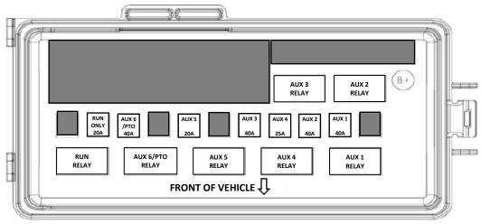
Max Combined Fuse "rating" allowed for Aux Swit hes 1,2,3,4,5, 6/PTO and Run Only is 225A. These Aux/PTO/Run fuses can be relocated to accommodate the loading on them. The maximum allowable total continuous amperage is 135A. Maximum fuse rating in any one location is 40A.
