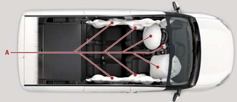
**A SEVEN STANDARD AIR BAGS<sup>[5]</sup>** raise Ram ProMaster City Wagon to top-tier consideration: few competitive vehicles in the class offer so many. These include dual-stage driver and front-passenger air bags; side air bag inflatable curtains; front seat-mounted thorax air bags; class-exclusive<sup>[1]</sup> driver's-side knee air bag; to all of that, add dual front seat belt pretensioners and seat belt load limiters.
