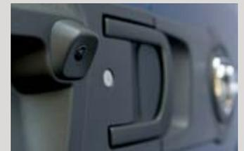
**D THE PARKSENSE® REAR PARK ASSIST SYSTEM<sup>[6]</sup>** is packaged with the ParkView Rear Back-Up Camera.<sup>[6]</sup> It's activated by pushing the Reverse gear selector and operates below 5 mph, using audible warnings to alert the driver if there are obstacles to the rear. Chimes in the display cluster increase in intensity as the vehicle nears the obstructions.
