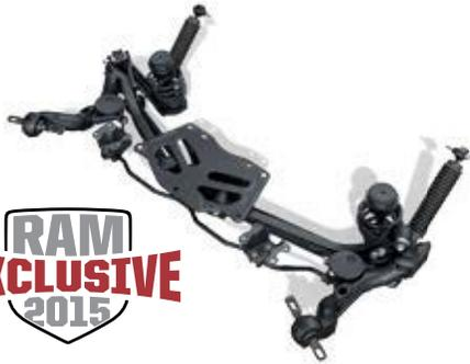
**THE RAM PROMASTER CITY™ BI-LINK REAR SUSPENSION** is a category-unique asset that delivers outstanding driving comfort, enhanced stability, benchmark handling with remarkable confidence. Steel, cargo-rated coil springs supply high-fatigue durability; muscular telescopic twin-tube hydraulic shocks are designed for minimal mass and maximum performance. A 16-mm solid stabilizer bar with optimized torsional stiffness also enhances durability.
