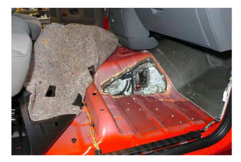
6. You are now able to install and assemble the PTO and pump through the opening. Note: larger pumps must be inserted through the hole and moved toward the rear of the opening before installing the PTO. The pump is then slid forward to connect to the installed PTO.
